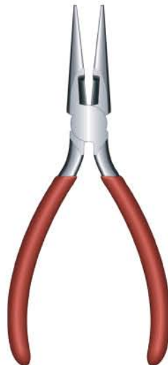
pince F à long bec M needle-nose pliers alicates M de punta F Spitzzange F pinza F a becchi M lunghi
